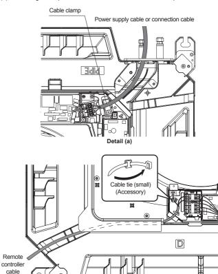
(4) Replace the Control box cover and Wiring cover. Securely tighten the screws.
