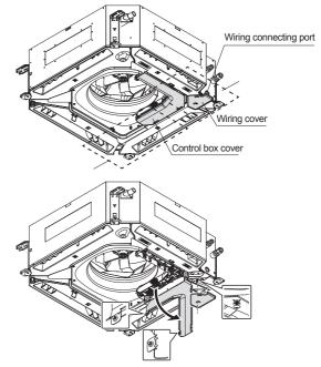
(2) Thread each cable through the holes or indents of the cabinet and connect the wires.
