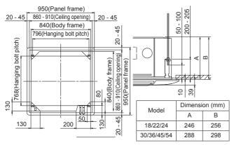
• Refrigerant piping and drain piping positions.
