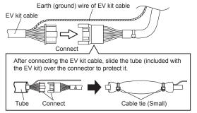
When you attach the cable clamp, make sure that the cables are not jutting out from the clamp or being pinched by the clamp.
