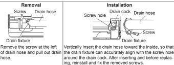
Installing the drain cap
