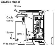
(3) Connect the end of the connection cable fully into the terminal block. 004/007/009 model
