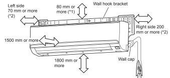
The distance between the wall hook bracket and the ceiling. \*1.
