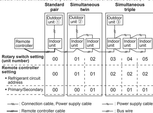
\* Make sure that the indoor unit with the unit number 00 is connected to the outdoor unit using a connection cable.
