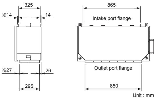
※ Spacing between flange and drain pan.
