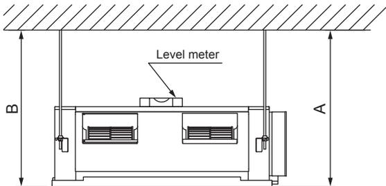
The side A of the unit with the drain port should be slightly lower than the opposite side B of the unit. The height difference between sides A and B should be from 0 to 20mm.
